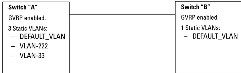
The **show vlans** command lists the dynamic (and static) VLANs in switch “B”.
