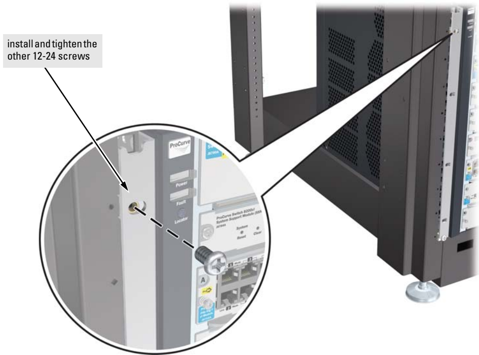
Figure 2-5. Screws in Bracket Being Installed
