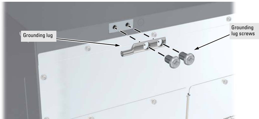
Figure 2-11. Attaching Grounding Lug to the 8200zl Switch
